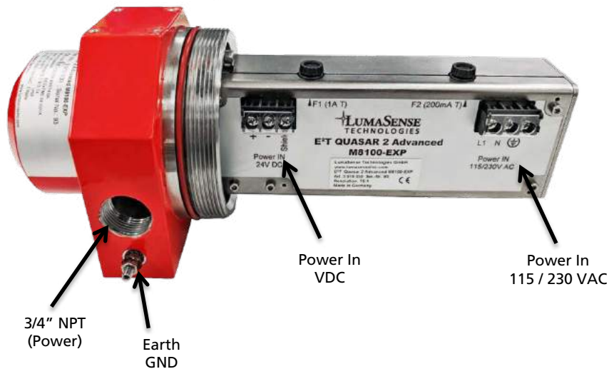
Figure 7: Input Terminals of the E 2 T QUASAR 2 M8100-EXP.
