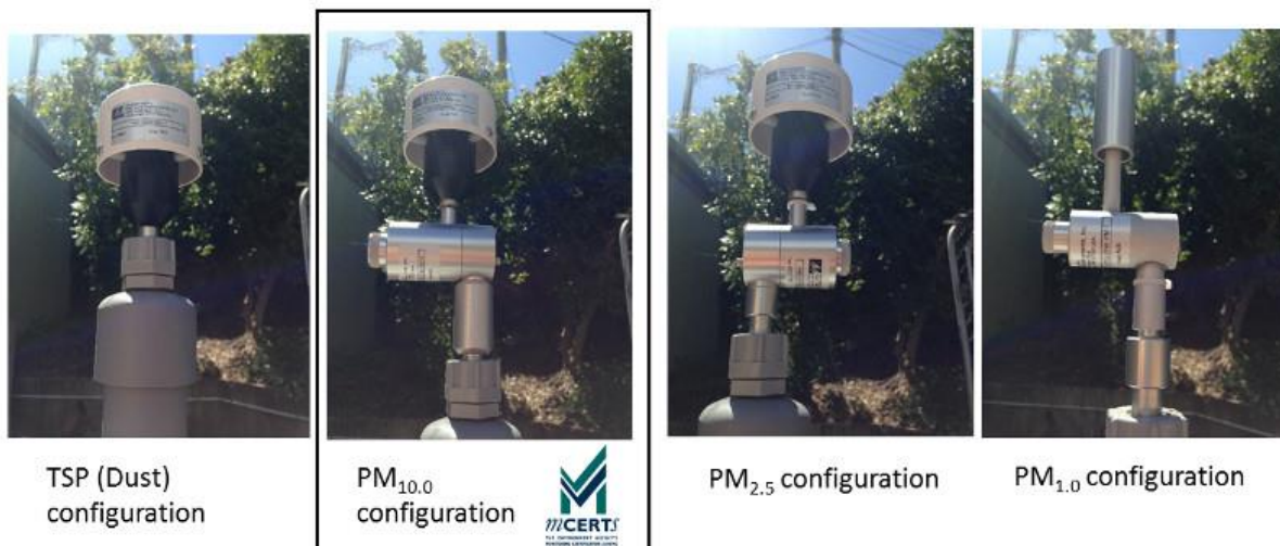
Figure 1-12 Size selection in the Particle Monitor is determined by the sharp cut cyclone on the inlet
