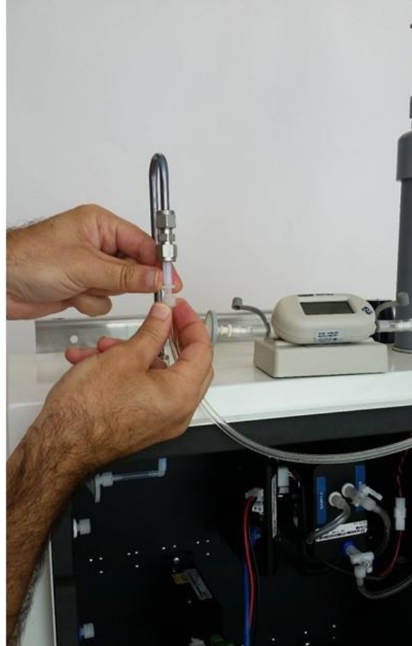
Figure 4-5 To measure the flow rate, remove the inlet filter and attach the inlet flow adaptor.
