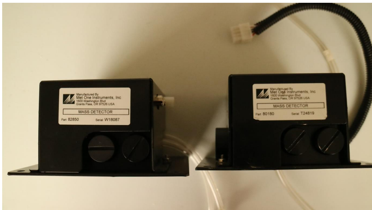
Figure 1-13 Left: 82850 optical module, Right 80180 optical module, the size and form factor are identical
