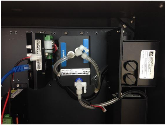
Figure 2-4 With mains power on, and with the 12 V DC fuse pulled out, there should be air flow coming from the top of the AQM as shown on the right. Disconnect the power (red/back) cable from the PM pump module while testing the power, as shown on the left
