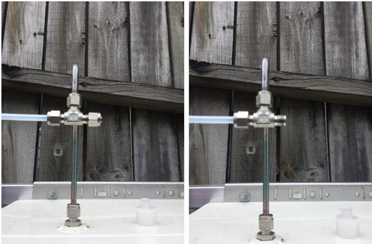
Figure 7-2 Left: Closed tee used with demand flow regulator. Right: Open tee used with fixed flow regulator.
