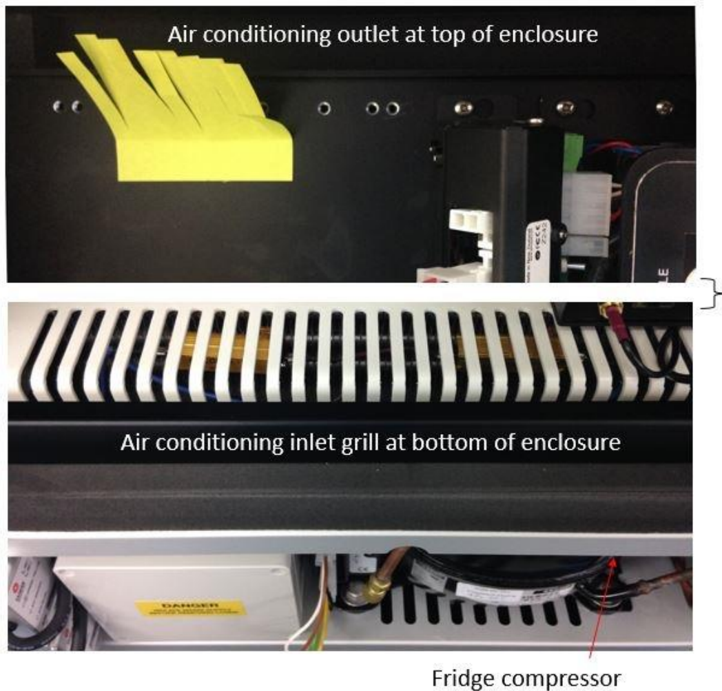
Figure 1-20 Air conditioned air is constantly circulated in the AQM 65 enclosure. Air comes in to the enclosure at the top and exits through vents at the bottom
