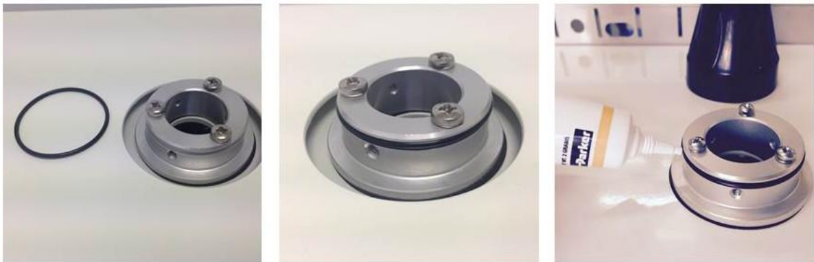
Figure 2-6 Add the O-ring and a small amount of lubricant.
