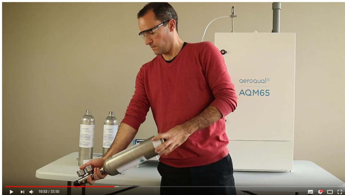
Figure 5-9 Calibration of Ox Ozone system for NO 2 YouTube: www.youtube.com/watch?v=InK1x7mTTQw
