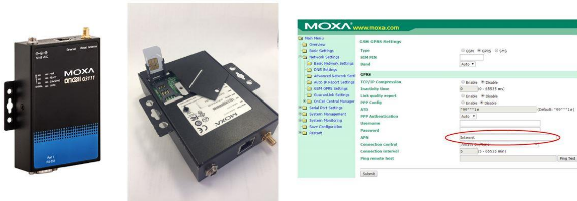
Figure 3-6 The MOXA modem uses a SIM card and it must be configured for use with the AQM 65
