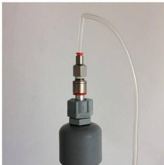
Figure 4-10 When checking the flow rate of the Particle Monitor (left) place the flow measurement adaptor above the cyclone. The position of the flow adaptor when measuring the Particle Profiler is shown on the right.
