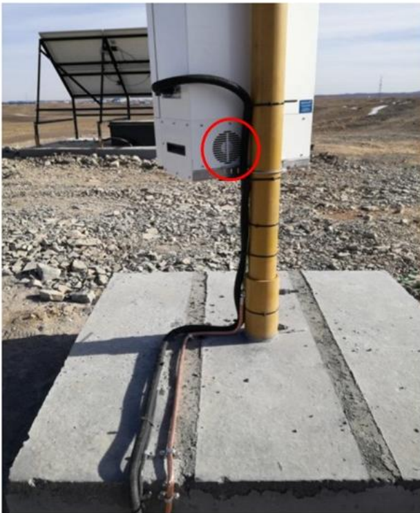
Figure 2: It is very important to maintain good air flow underneath the AQM 65. The temperature and relative humidity sensor is placed on the bottom plate (right) The AQM 65 should be mounted on an open bottom stand so that air can flow underneath the AQM 65, the cooling fan at the back (left) must also be unobstructed.
