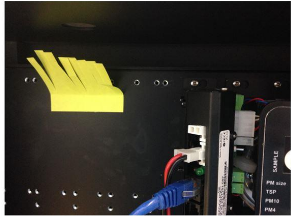
Figure 2-4 With mains power on, and with the 12 V DC fuse pulled out, there should be air flow coming from the top of the AQM as shown on the right. Disconnect the power (red/back) cable from the PM pump module while testing the power, as shown on the left
