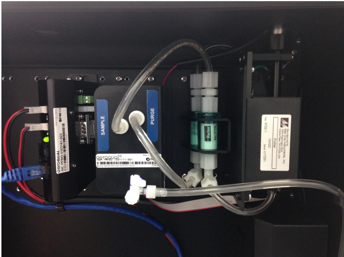
Figure 1-16 The Particle Profiler uses three modules: a) the optical module on the far right, b) the pump module in the middle, c) the electronics module on the left. The image above is the arrangement prior to July / August 2018.
