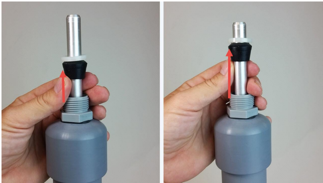
Figure 2-8 Create more length to the inlet by sliding the black rubber grommet up the tube.
