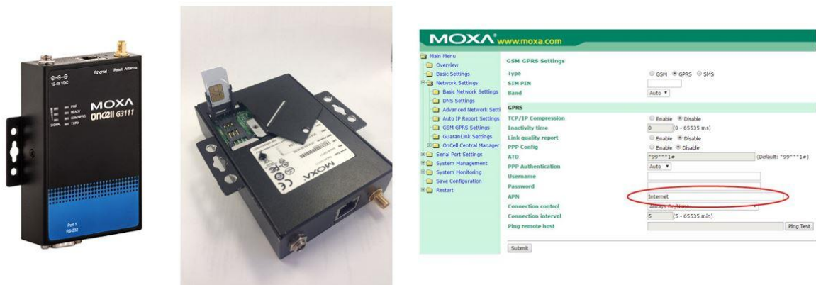
Figure 2-13 A SIM card must be inserted in to the modem and the Modem must be configured
