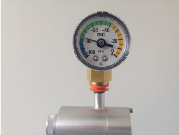
Place gauge on inlet above cyclone
