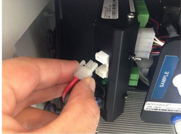
Remove power cable from electronics module
