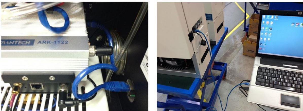
Figure 3-5 To establish a direct connection, a laptop must be connected to the ePC using an Ethernet cable
