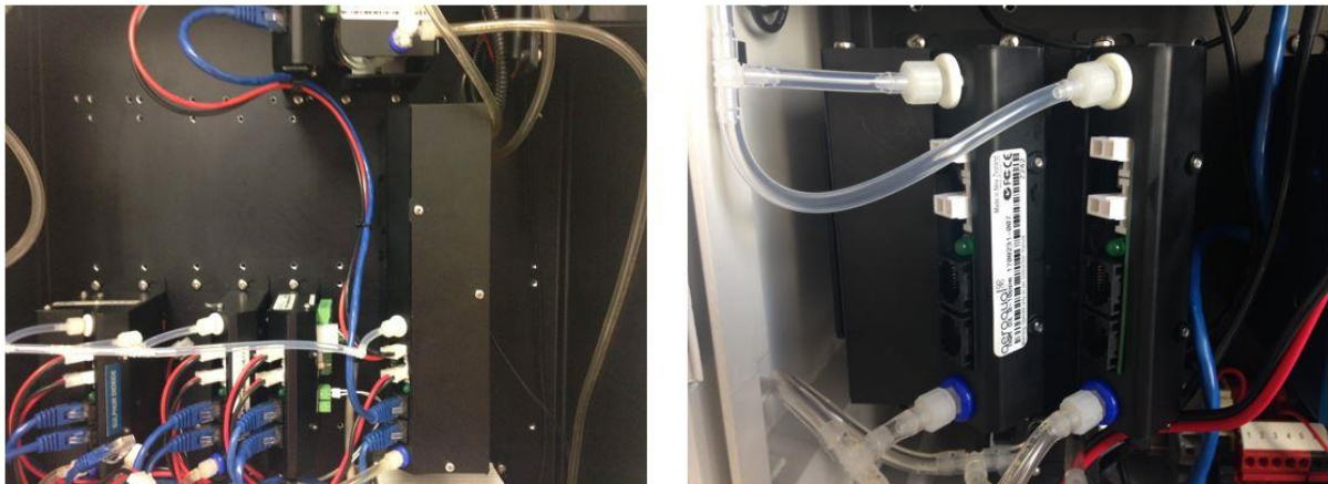
Figure 1-6 Left: The large size direct NO 2 measurement module, Right: Ox/O 3 system for measuring NO 2
