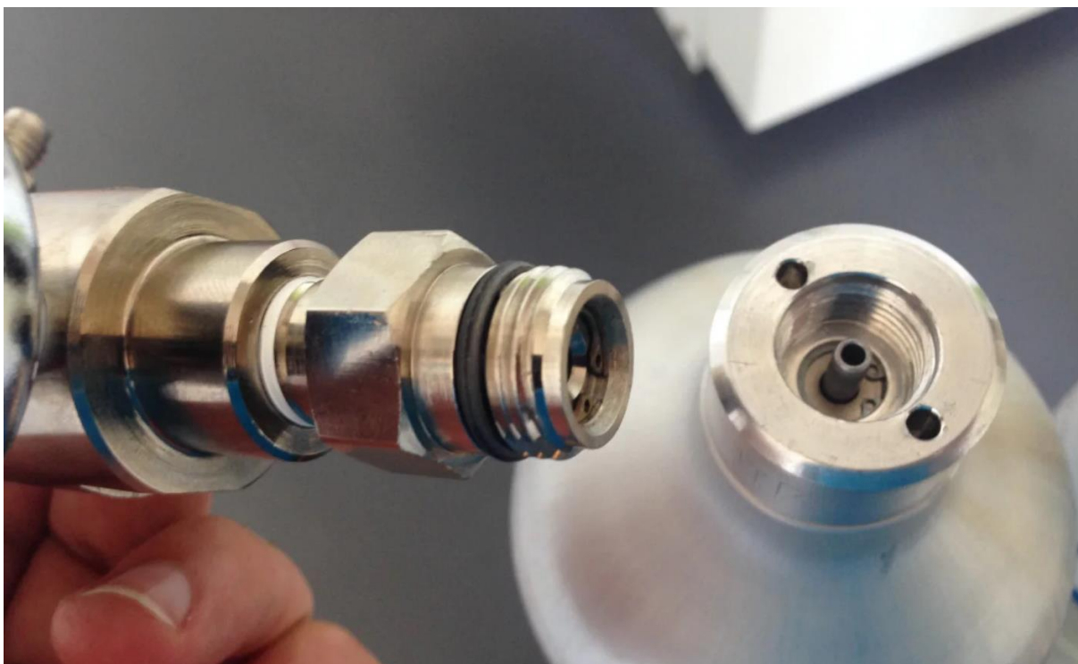
Figure 5-2 See the Aeroqual online training on connecting your gas regulator to your cylinder, Aeroqual YouTube channel.
