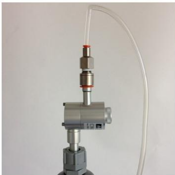
Figure 4-10 When checking the flow rate of the Particle Monitor (left) place the flow measurement adaptor above the cyclone. The position of the flow adaptor when measuring the Particle Profiler is shown on the right.
