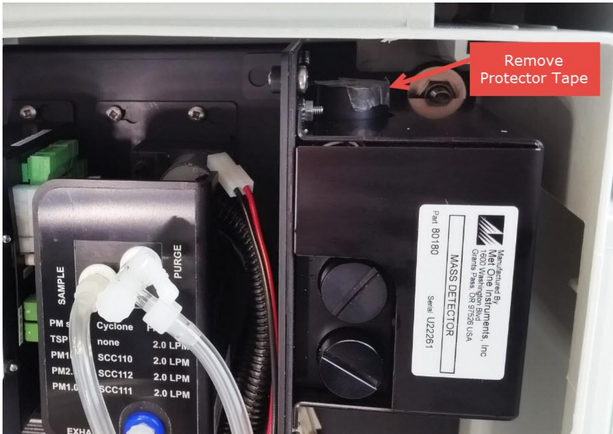
Figure 2-5 Remove the protective tape from the PM inlet
