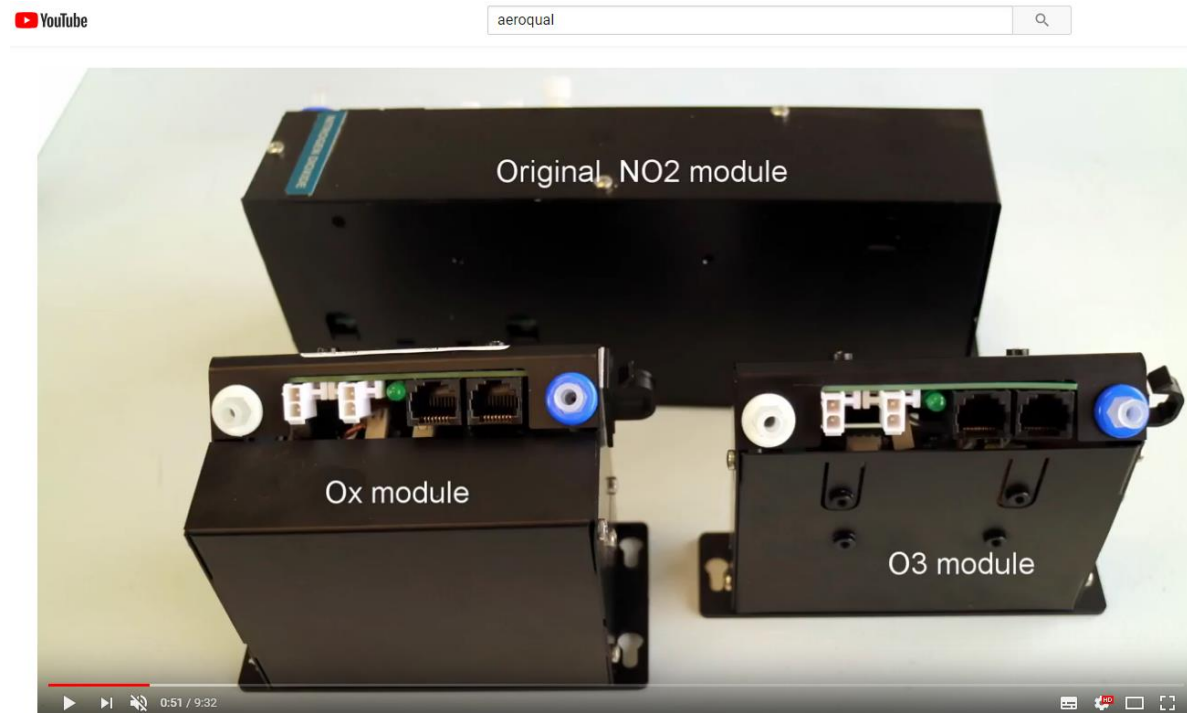
Figure 1-5 Replacing NO 2 module with O x /O 3 system for measuring NO 2 www.youtube.com/watch?v=4GS7ey4S-68
