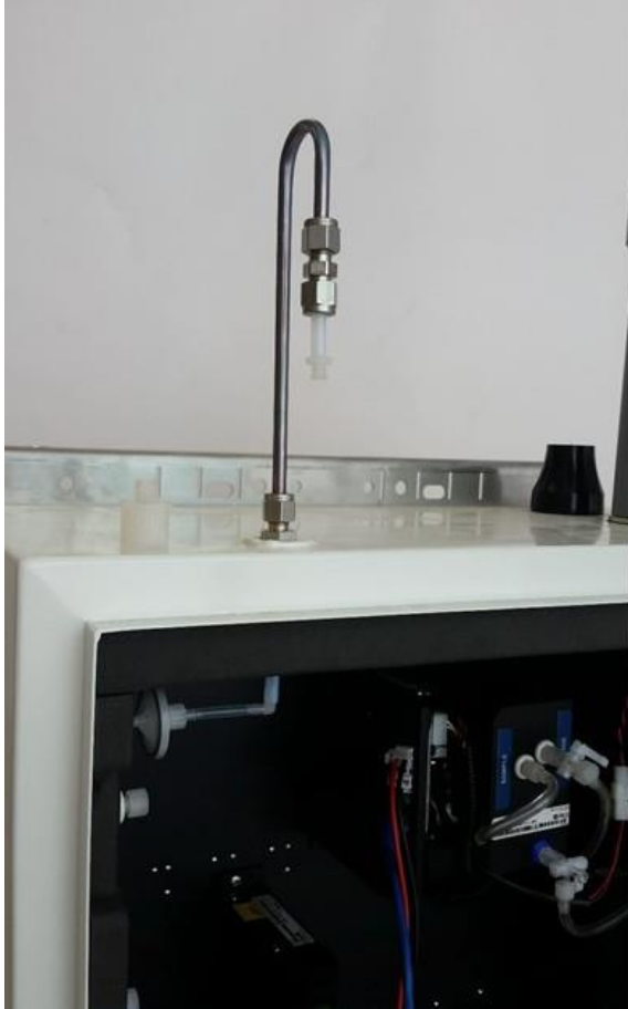
Figure 4-5 To measure the flow rate, remove the inlet filter and attach the inlet flow adaptor.
