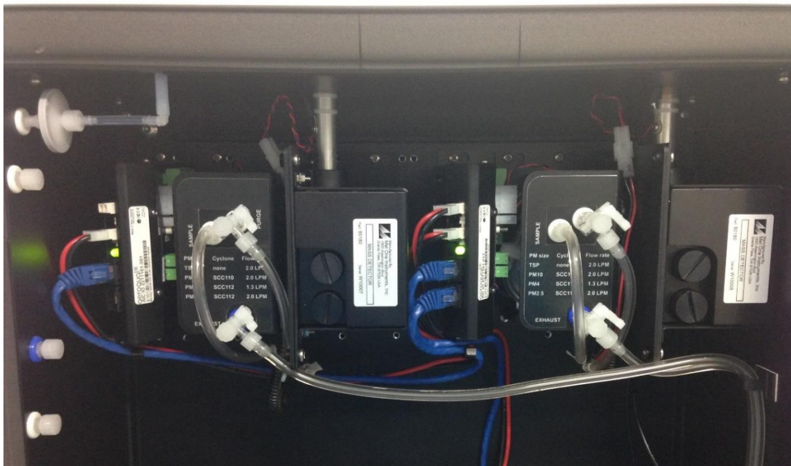
Figure 1-11 Two Particle Monitors can be installed in an AQM 65, each Particle Monitor will have three modules each
