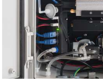
Inlet filters ensure hygiene and integrity of gas sample.
