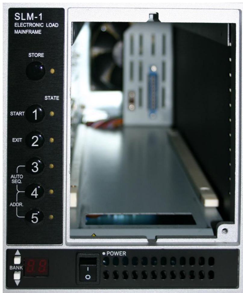
Figure 3-1 SLM-1 Chassis Front Panel, without Module
