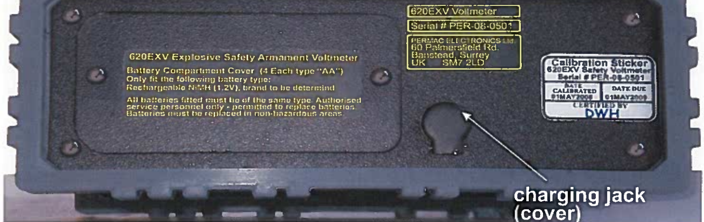
620EXV "No-Volts" Safety Voltmeter rear panel photo
