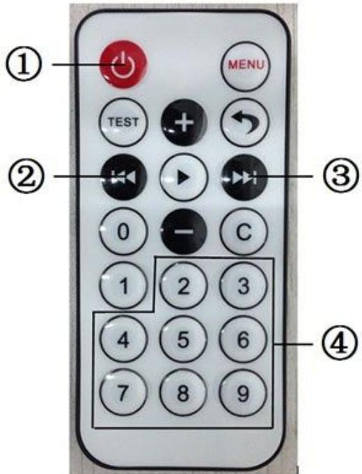
① On/Off ② Reduce duty ratio ③ Enlarge duty ratio ④ Frequency : 2→1Hz, 3→3Hz, 4→5Hz, 5→8Hz, 6→10Hz, 7→20Hz, 8→30Hz, 9→50Hz
