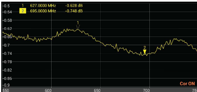
Figure 31 Interpreting Cable Loss Measurement
