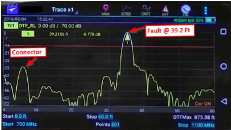
Figure 1 Typical Fault Location Measurement
