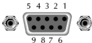
Figure 1 - RS-232 Connector Pinout
