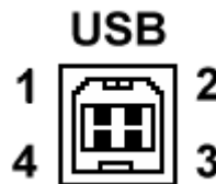
Figure 3-3: USB Connector pin orientation.
