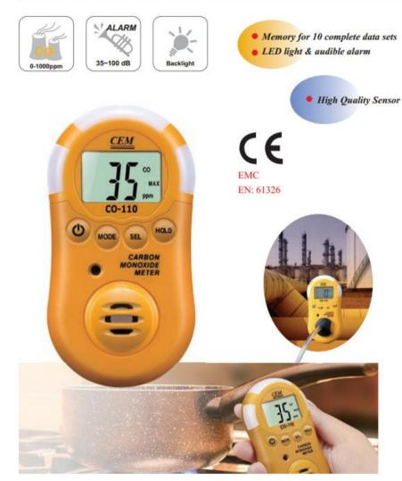
CO-110 Carbon Monoxide Meter detects the presence of carbon monoxide (CO) and measures concentrations between 1-1000 parts per million (PPM). The Meter indicates the presence of CO by a reading on the LCD and a beeper tone. The beeper function much like clicking of a Geiger counter: Above 200 PPM, the beeper sounds continuously with the concentration of CO. From 35 PPM to 200 PPM, the beeper sounds discontinuously with the concentration of CO.
