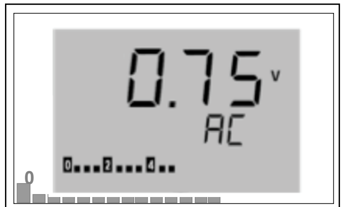
Figure 9. AC voltage display
