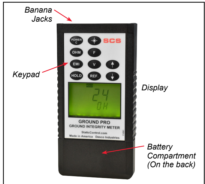
Figure 2. Ground Pro Meter features and components
