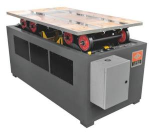
4. Customers are only requested to place the transport simulation tester on flat marble or concrete ground. No special foundation is needed during installation.
