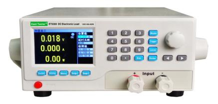
ET53 series DC programmable electronic load provides 1mV/10mV, 1mA/10mA high resolution and precision with superior performance. It is equipped with 12 common modes and complete test functions, which can be widely used in charger, switching power supply, linear power supply, battery and other production line testing.
