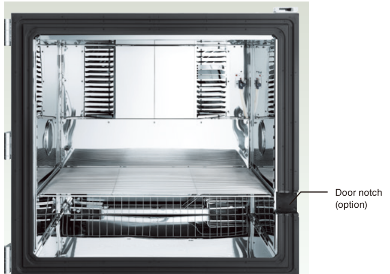
Inside of the ARS-1100-5 chamber
