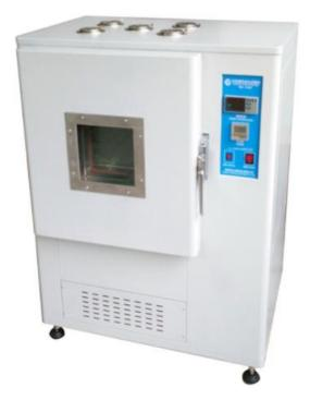
It is mainly used for hot air aging test of rubber and plastic products, electrical insulation and other materials. It detects changes in aging extension and tension resistance of products and materials. PID automatic adjustment temperature controller can set operating temperature arbitrarily and automatically adjust temperature.
