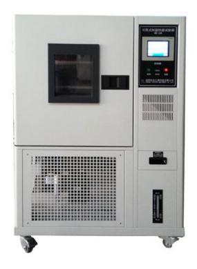
It mainly tests the heat resistance, cold resistance and moisture resistance of various materials. It is a testing device for simulating the storage, transportation and use environment of parts or materials of electricians, electronics, instruments and other products under various environments.
