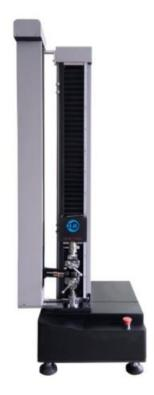
It is used in the testing of mechanical properties such as tensile, compression, bending, shearing and peeling of materials. It is mainly used in various industries to perform tensile strength testing on materials and is suitable for laboratory applications.
