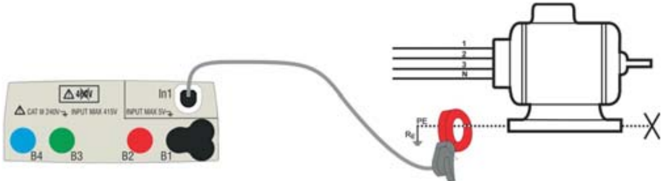
Fig. 27: Direct measurement of leakage current in three-phase systems
