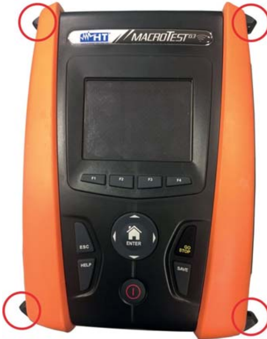
Fig. 41: Instrument with fitted half-shells and hooks
