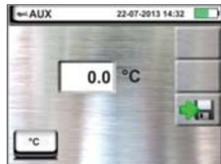
Fig. 33: Measurement of environmental parameters through external probes
