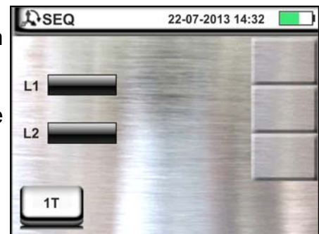
Fig. 23: Phase sequence check of 2T phases with terminal and remote lead
