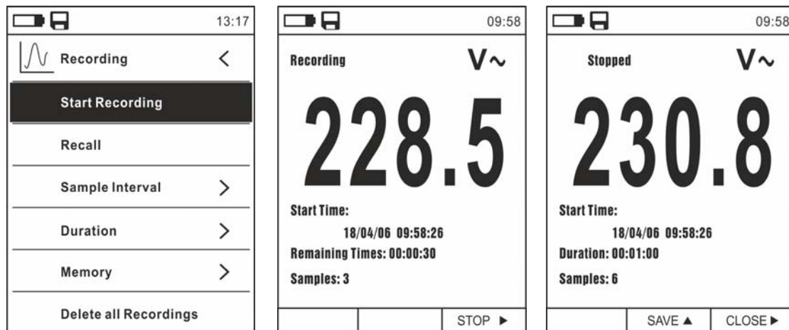
Fig. 33: Data logger function – Starting and stopping recording
