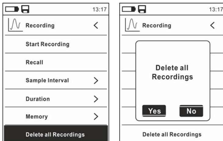
Fig. 38: Data logger function – Deleting all recordings
