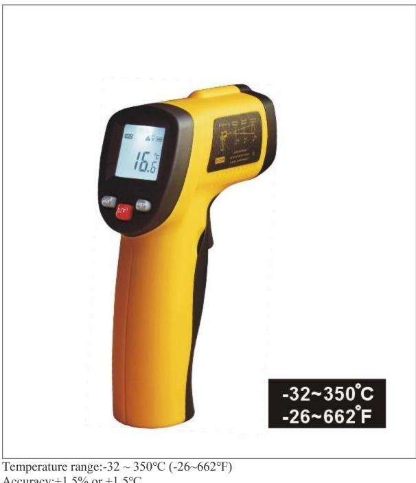
Temperature range: $-32 \sim 350^{\circ}$ C ( $-26 \sim 662^{\circ}$ F) Accuracy: $\pm 1.5\%$  or  $\pm 1.5^{\circ}$ C Repeatability: $\pm 1\%$  or  $\pm 1^{\circ}$ C Distance Spot Ratio:12:1Emissivity:0.95 preset Resolution:0.1°C/°F Response Time:500ms Wavelength:8-14µm °C/°F Selection Data Hold function Laser Target Pointer selection Backlight ON/OFF selection Auto Power Shut Off Power supply:9V battery Weight:147.5g(Including battery) Dimension:153\*101\*43mm Packing Method:Blister+Card
