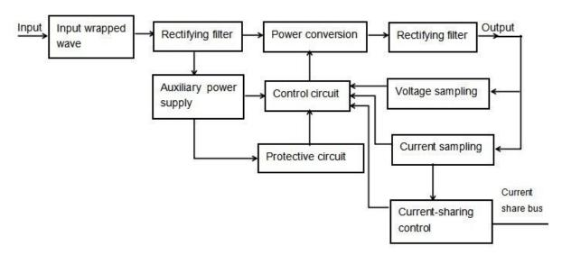
Output constant voltage and current are sampled by output side, ensure high stability and reliability.
