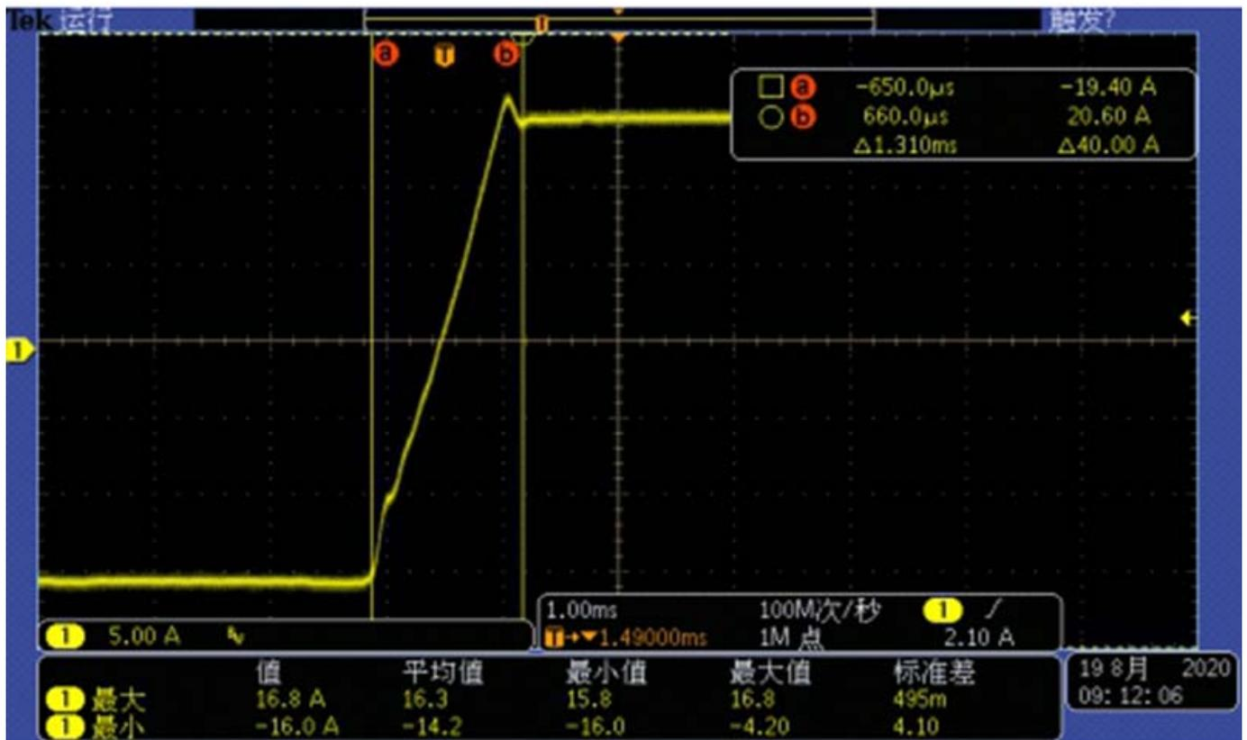
Single module reverse 15A to forward 15A switching waveform (switching time < 1.4mS)
