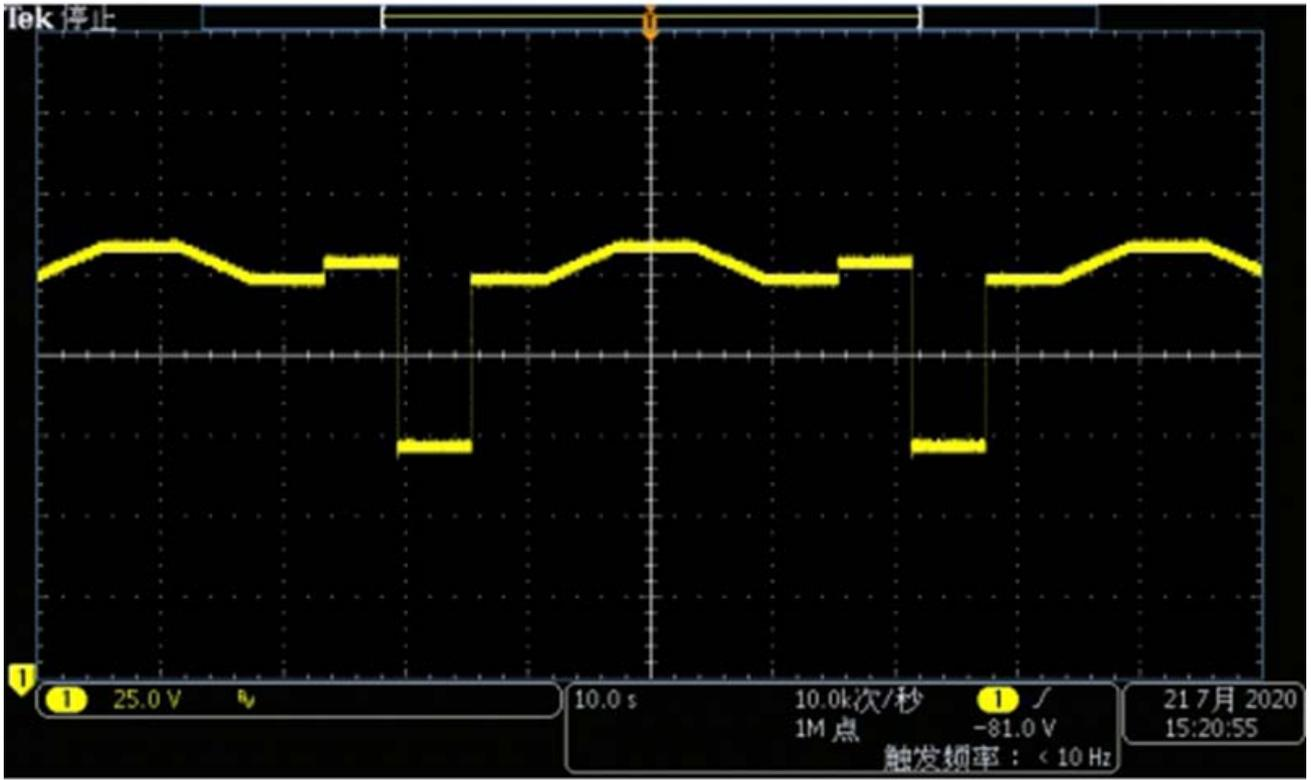
LV123 working range upper limit test waveform
