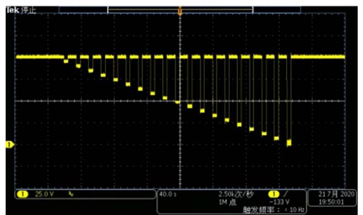
ISO-16750-2-4.6.2 Voltage descent reset test waveform
