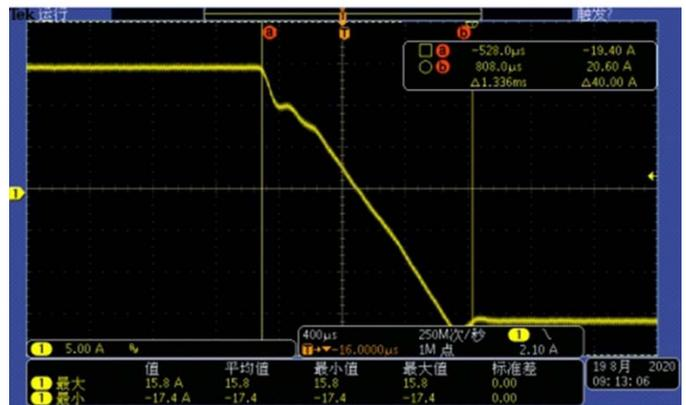
Single module forward 15A to reverse 15A switching waveform (switching time < 1.4mS)
