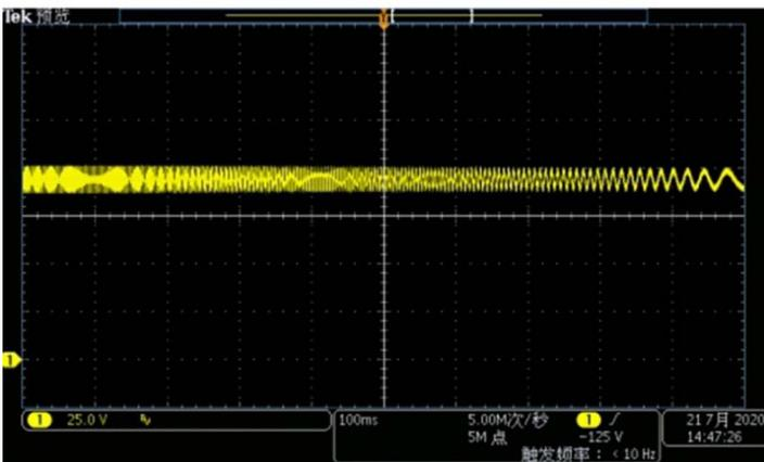
LV123 voltage ripple test waveform (ripple frequency range: 1HZ ~ 2KHZ)
