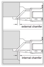
for internal chamfer measurement, diameter should be larger than ØD
