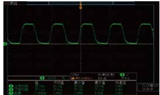
IT8906A-1200-240 5 kHz dynamic loading 0A-50A
