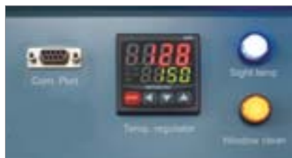
Electronic over temperature shutdown system.
