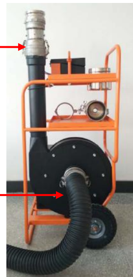
High flow Duct testing under Negative pressure
