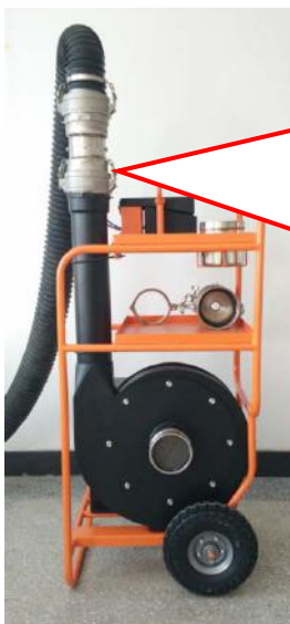
High flow Duct testing under positive pressure
