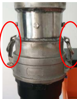
Cam lock adaptor in locked status.
