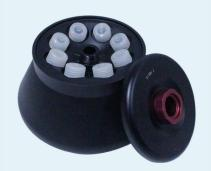
When the angle rotor is running, the centrifuge container and the rotating shaft form a fixed angle, and the sample is deposited at the bottom of the centrifuge tube and the side wall near the bottom.
