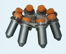
When the swing-out rotor is running, the basket is horizontal, at right angles to the rotating shaft, and the sample is deposited at the bottom of the centrifuge tube.
