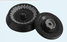
When the angle rotor is running, the centrifuge container and the rotating shaft form a fixed angle, and the sample is deposited at the bottom of the centrifuge tube and the side wall near the bottom.
