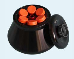
When the angle rotor is running, the centrifuge container and the rotating shaft form a fixed angle, and the sample is deposited at the bottom of the centrifuge tube and the side wall near the bottom.
