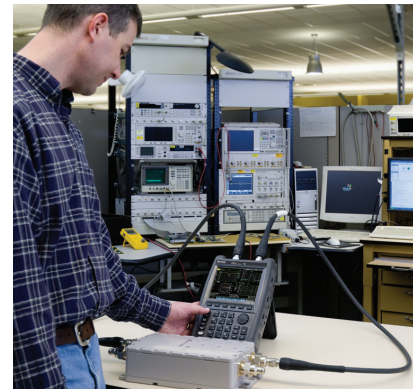
Tower mounted amplifier (TMA) measurement
