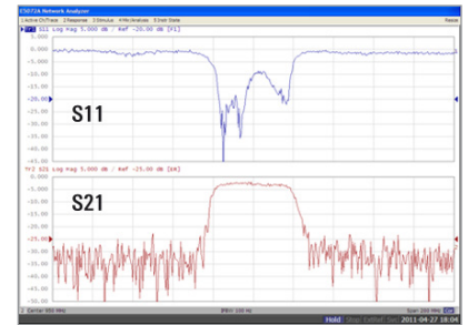
Figure 7. Accurate measurements with low signal input, Upper (power = -55 dBm with external 20 dB attenuator), Lower (power = -75 dBm with built-in attenuator)
