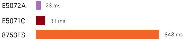
Figure 19. Measurement speed comparison: 1601 points, full 2-port cal, 1 GHz to 1.2 GHz IFBW = 6 kHz (8753ES), 500 kHz (E5071C and E5072A)
