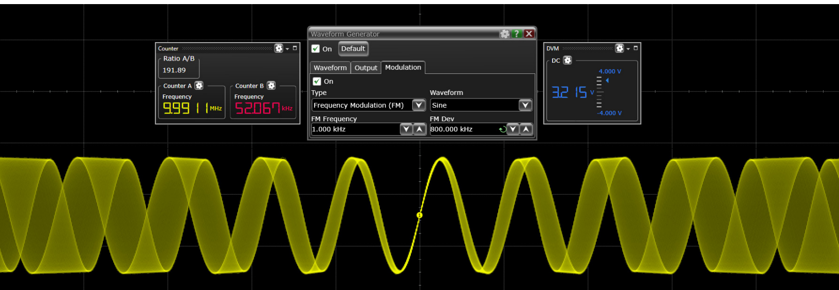
Generating a 10 MHz sine wave with frequency modulation, while measuring two signal frequencies with counters and a third signal's DC voltage with the DVM. Note that channels need not be enabled for the counter and DVM to operate.
