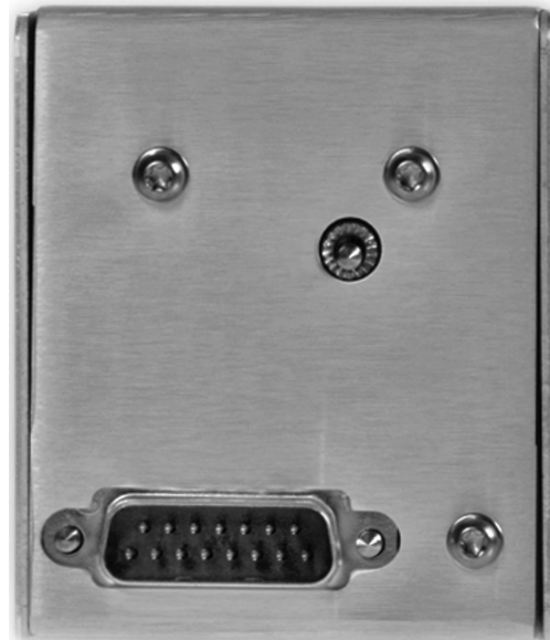
Pulse I/O adapter (N1966A) simplifies connections
