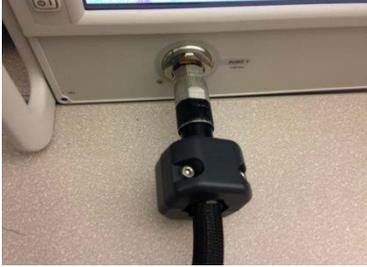
4. Position the cable clamp over the nut that secures the PNA/PNA-X port connector to the front panel such that the flat areas of the cable clamp align and lock onto the flat areas of the nut. The cable clamp should not rotate freely.
