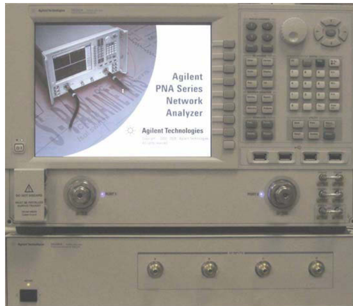
Figure 1 N5242A 2-Port PNA-X with N5280A
