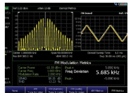
Characterize AM/FM signals using AM/FM demodulation
