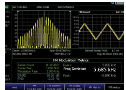
Characterize AM/FM signals using AM/FM demodulation
