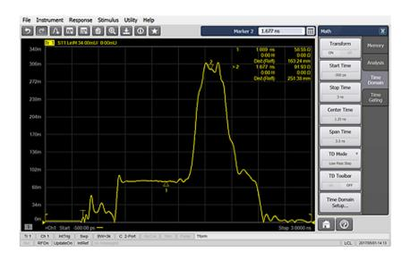
The S97010B time domain analysis capability allows you to measure the time domain response of a device. The analyzer can transform frequency domain data to the time domain or time domain data to the frequency domain.
