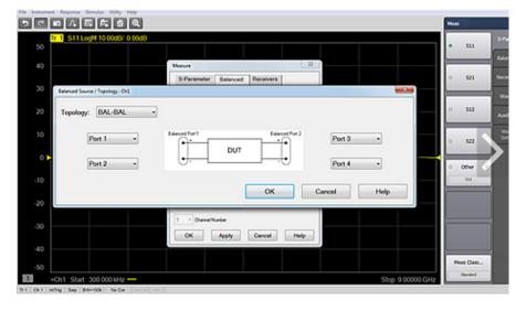
The S97551B software enables full multiport error correction and measurement capabilities when using multiple USB vector network analyzers
