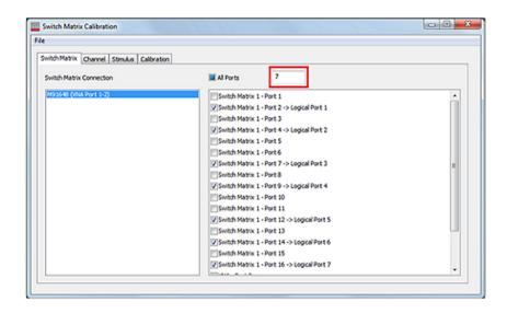
This application provides a macro which enables full multiport error correction and measurement capabilities using external switch instruments
