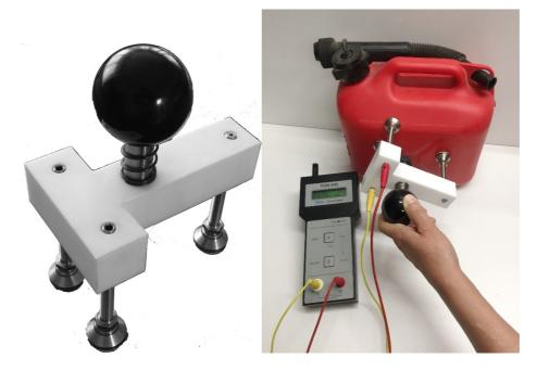
Up to now, surface resistances have been measured with heavy weights as defined in the relevant standards (e.g. standards group DIN IEC/TS 61340 and IEC/TS 60079). The measurement setup generally provides for a horizontal setup to ensure the pressure of the defined weights. Such measurements are usually performed in laboratories. In the ongoing production process and to ensure product quality, the prescribed measuring arrangements cannot usually be implemented.
