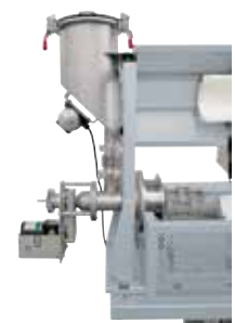
Vibration generator at the charging funnel for improved powder supply
