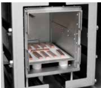
Heat treatment of copper bars under hydrogen in VHT 08/16 MO
