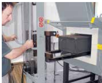
Working with protective gas boxes for a protective gas atmosphere using a charging cart
