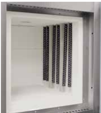
Vertically mounted SiC rods
