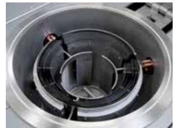
Cylindrical retort with tungsten heating
