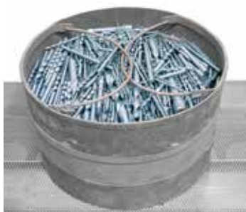
Blueing of drills in water steam atmosphere in a furnace of the NRA range
