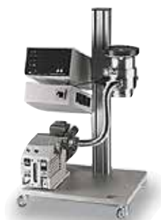
Vacuum pump stand for operation up to 10 -5 mbar
