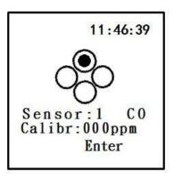
Press "↑" or "\ " key to select the sensor need to calibrate, then, press "↑" or " key to select "Enter" to confirm the zero calibration. The zero calibration for this sensor is finished.
