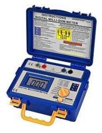
Milliohm Meter PCE-MO 2002 (Milliohm Meter with ruggedized and waterproof carrying case. With highly accurate measurement range)
