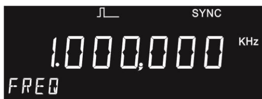
Figure 4-4 Generate a Pulse Wave
