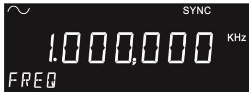
Figure 4-1 Generate a Sine Wave
