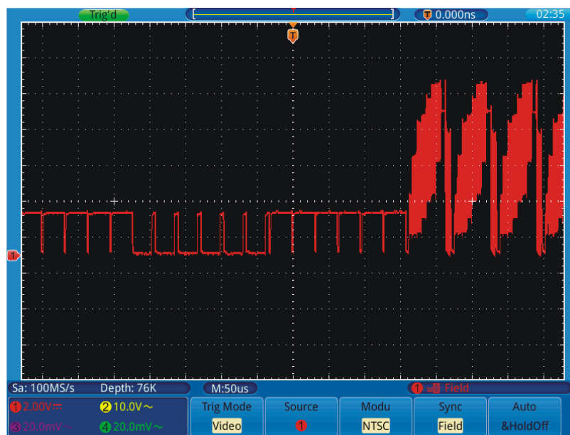
Figure 50. Waveform Captured from Video Field Trigger.
