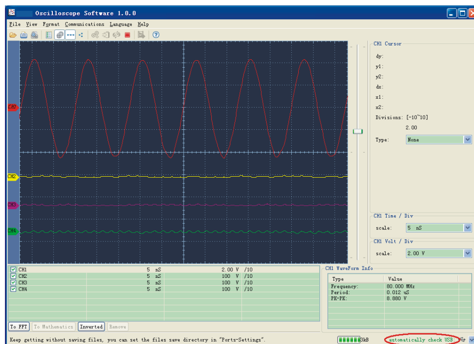
Figure 37. Connect with PC through USB port.
