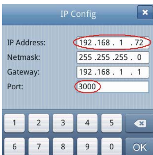
Figure 40. Set the network parameters of the oscilloscope.
