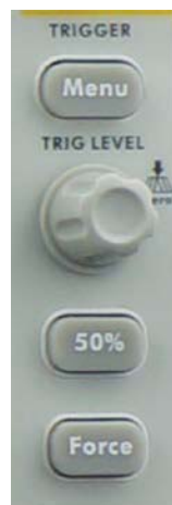
Figure 12. Trigger Control Zone.
