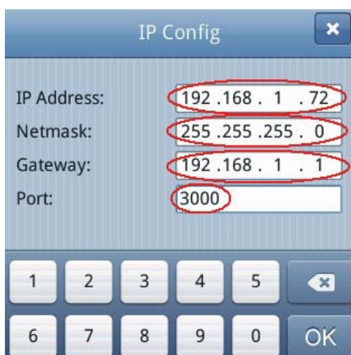
Figure 43 Set the network parameters of the oscilloscope.
