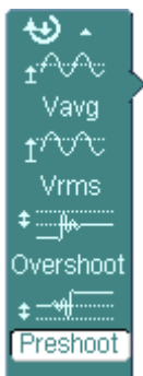
Figure 2- 125 Table 2- 80 The Voltage Measurements menu (Page 3/3)
