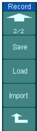
Figure 2- 107 Table 2- 70 The Storage menu when the save as external memory
