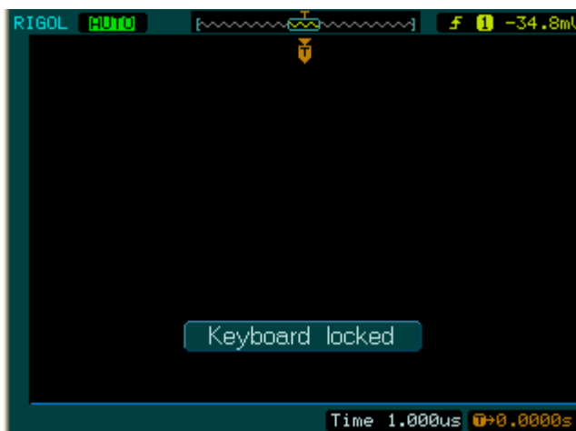
Figure 2- 118 Interface of keyboard locked
