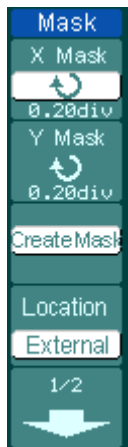
Figure 2- 96 Table 2- 60 The Mask setting menu (Page 1/2)
