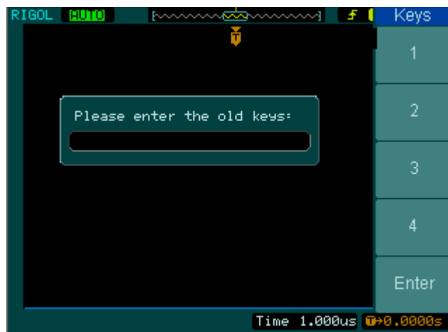
Figure 2- 120 Interface of key resetting
