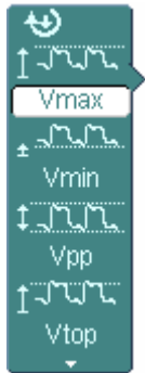
Figure 2- 123 Table 2- 78 The Voltage Measurements menu (Page 1/3)
