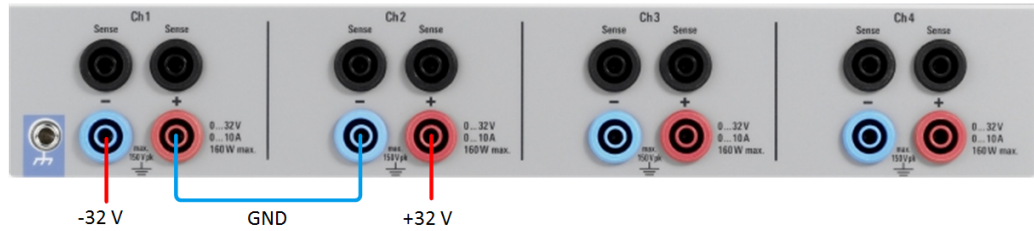
Figure 5-5: Example of a multi-quadrant connection
