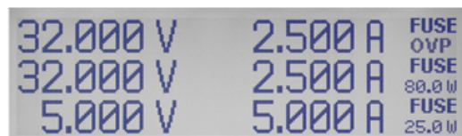
Figure 4-6: Overvoltage protection (example R&S HMP2030)
